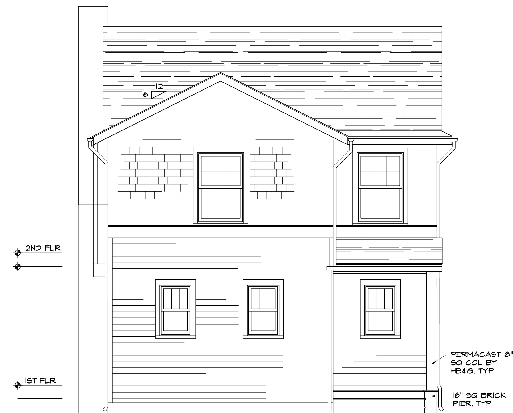
3 REAR ELEVATION (NORTH) SCALE: 1/4" = 1'-0"
