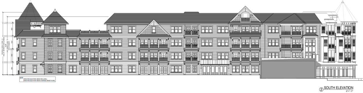
Illustration H.7. — South elevation of Condominium Building One showing Tuscan columns without plinths at the first floor (Sheet A-6).
