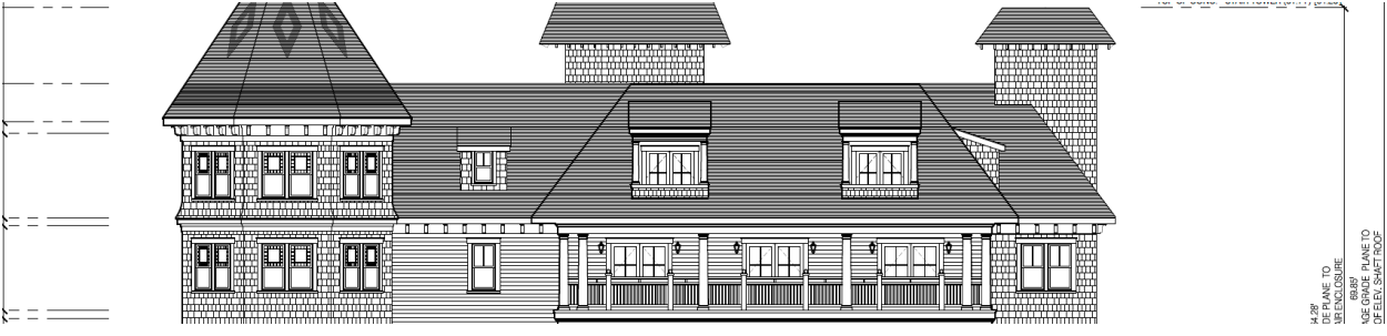
Illustration C.8.b. — Hotel dormers, east elevation, showing a single window dormer beneath a shed roof and two sets of double doors beneath shed roofs (Sheet A-11).
