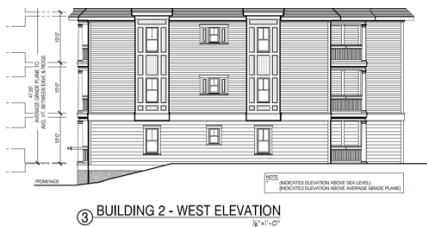
Illustration F.1.c. — West elevation of Condominium Building Two showing proposed clapboard reveal at first floor (wide) and upper floors (narrow) (Sheet A-8).
