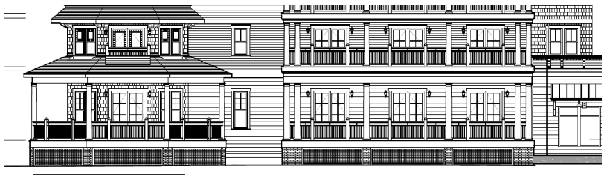
Illustration E.3.c. — First floor, east elevation of the Hotel showing inappropriate Colonial Revival windows (Sheet A-12).
