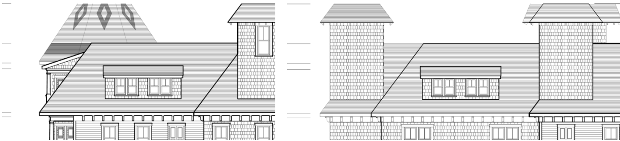
Illustrations C.11.a. and C.11.b. — The north and west elevations of the Hotel showing proposed, non-conforming, double dormers (i.e., pop-ups) (Sheet A-12).
