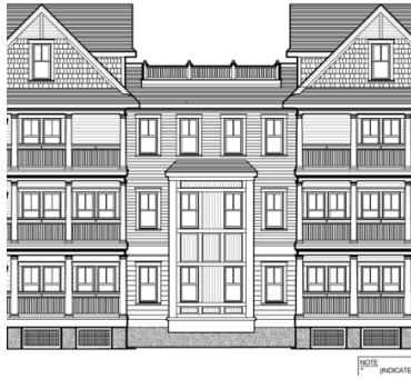
Illustration F.5.b. — Detail of north elevation, Condominium Building Two, showing paneled areas between widows on projection between balconies (Sheet A-8).
