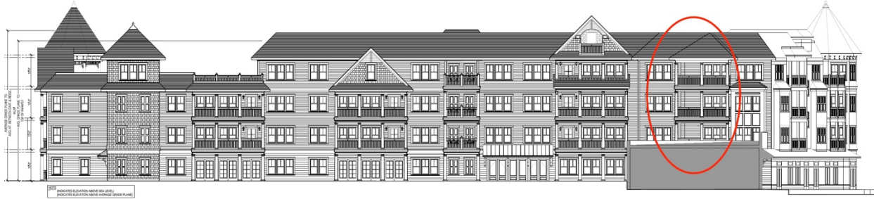
Illustration I.10. — South elevation of Condominium Building One showing balconies with no lighting indicated.
