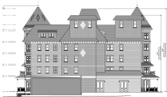
Illustration E.5. — North elevation of Hotel (Sheet A-12), showing upper staircase towers with two windows each.
