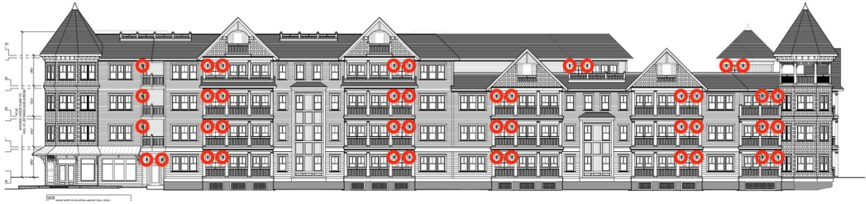
Illustration I.8.a. — North elevation of Condominium Building One showing lighting (most of which entails two light fixtures flanking single doors onto balconies) (Sheet A-6).
