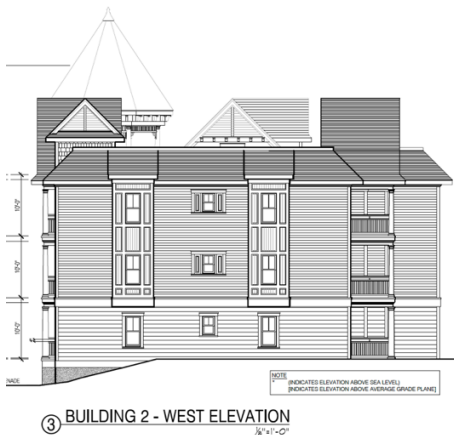
Illustration F.5.c. — Detail of west elevation, Condominium Building Two, showing paneled areas between widows on projections (Sheet A-8).
