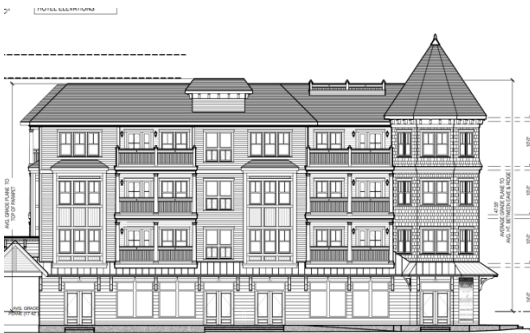
Illustration D.4. — East elevation of Condominium Building One (Sheet A-5) showing single balcony doors with non-conforming single side-light windows on each of the six balconies. These balcony doors should match single balcony doors on other elevations and should not include side-light windows.
