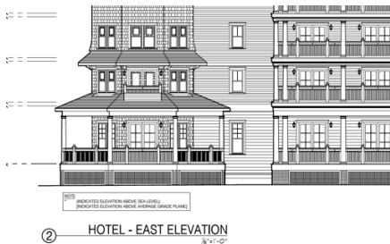
Illustration F.1.a. — East elevation of the Hotel showing proposed clapboard reveal at first floor (wide) and upper floors (narrow) (Sheet A-11).
