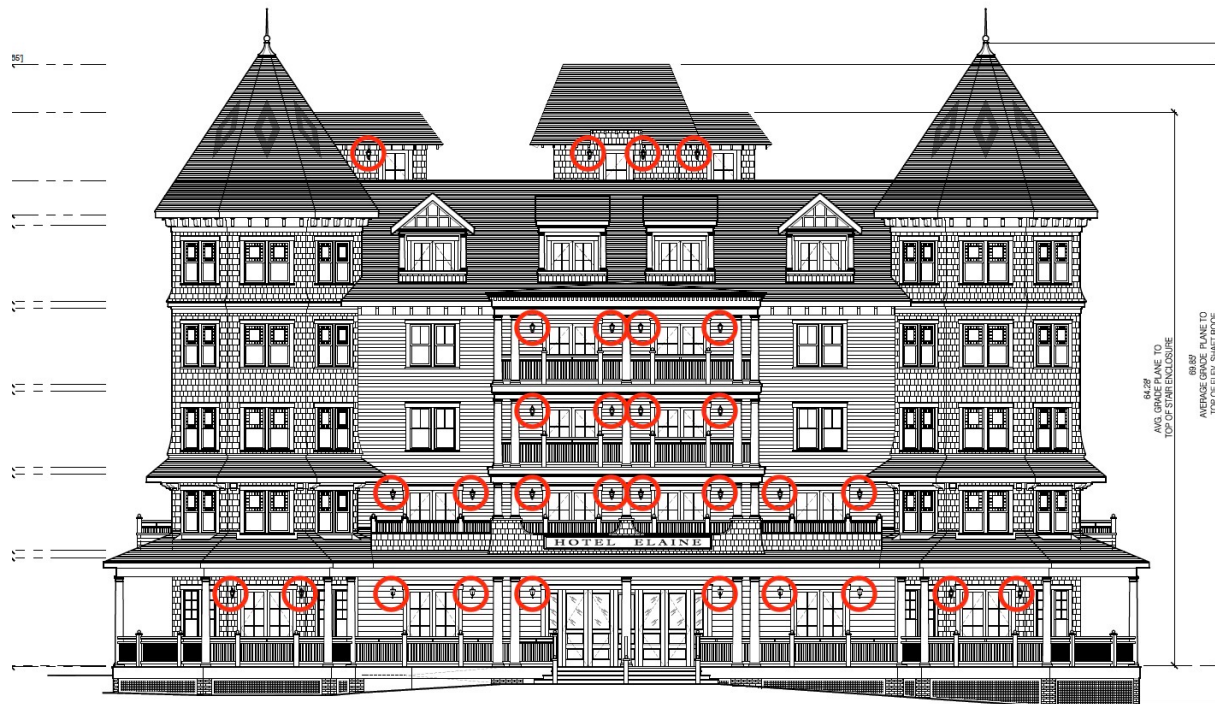
Illustration I.4.a. — South elevation of the Hotel showing thirty (30) proposed lantern fixtures (Sheet A-11).
